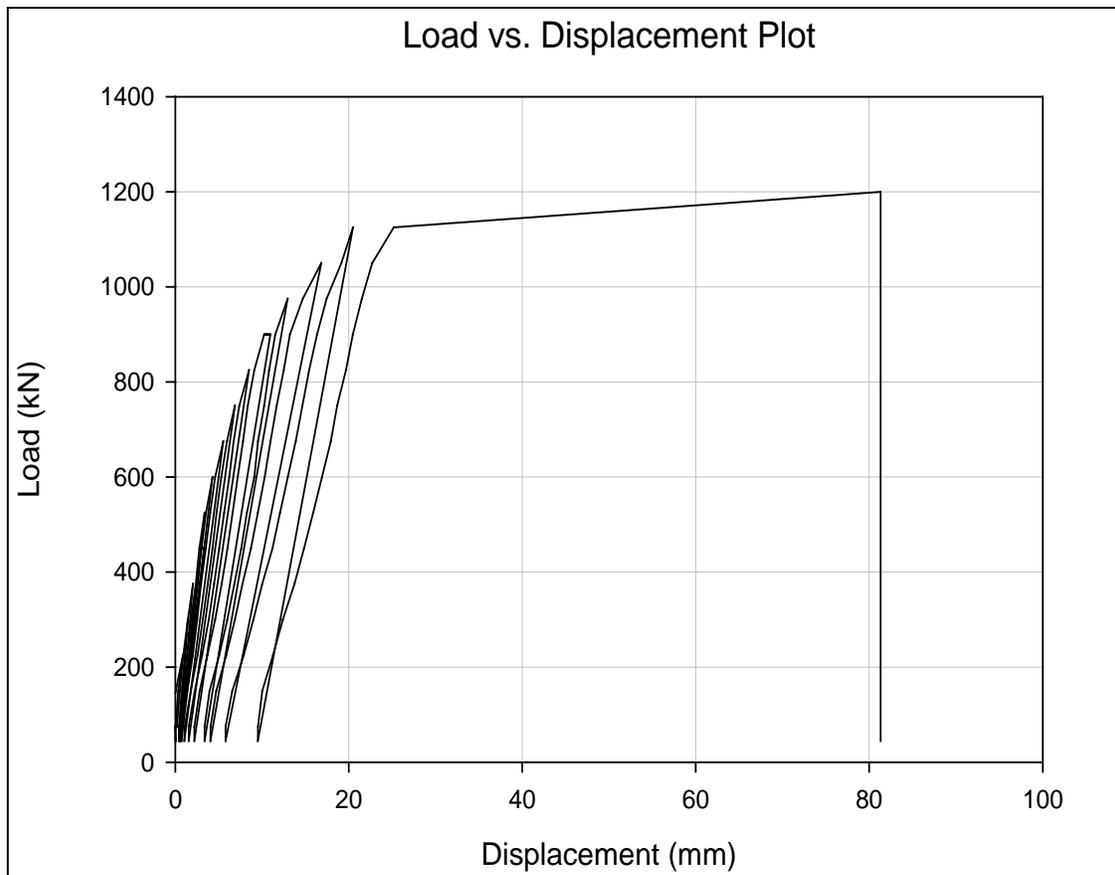
FIG. 3: Load vs. movement plot – Solaris sacrificial test micropile
