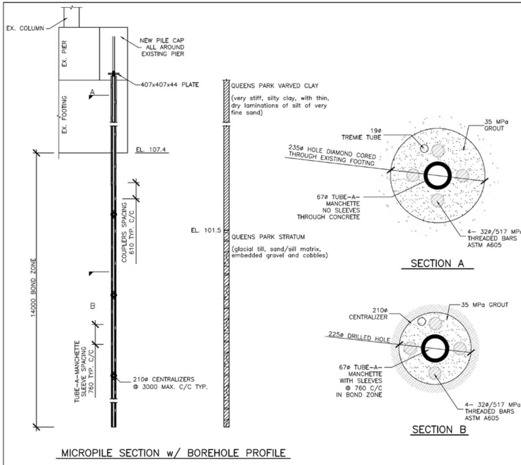
FIG. 1 Sacrificial pre-production micropile section and soil profile at the 130 Bloor W. project
