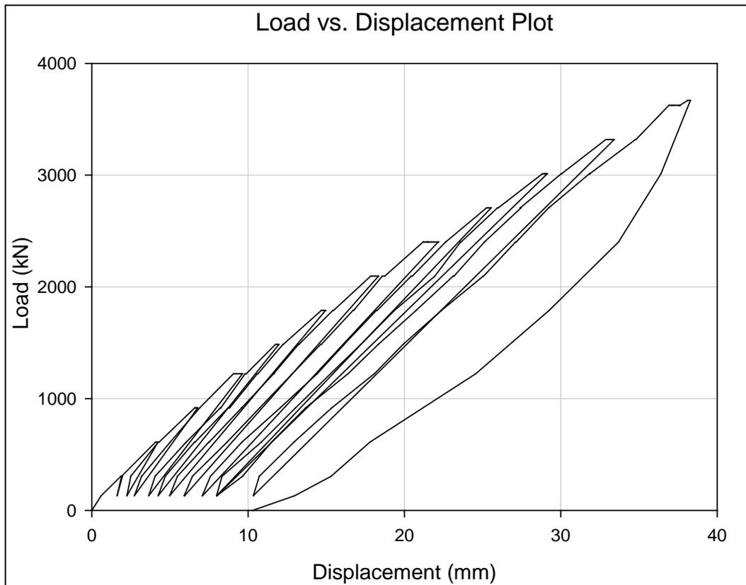
FIG. 4 Load vs. movement plot – Hullmark Centre sacrificial test micropile
