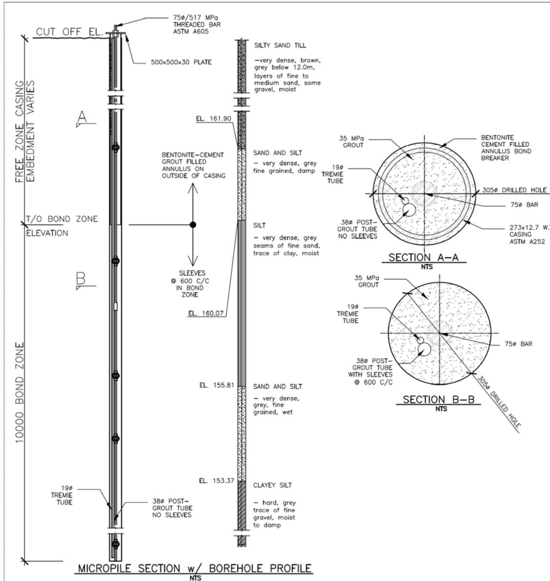
FIGURE 5. Hullmark Centre Project - Sub-surface profile and configuration of pre-production micropile
