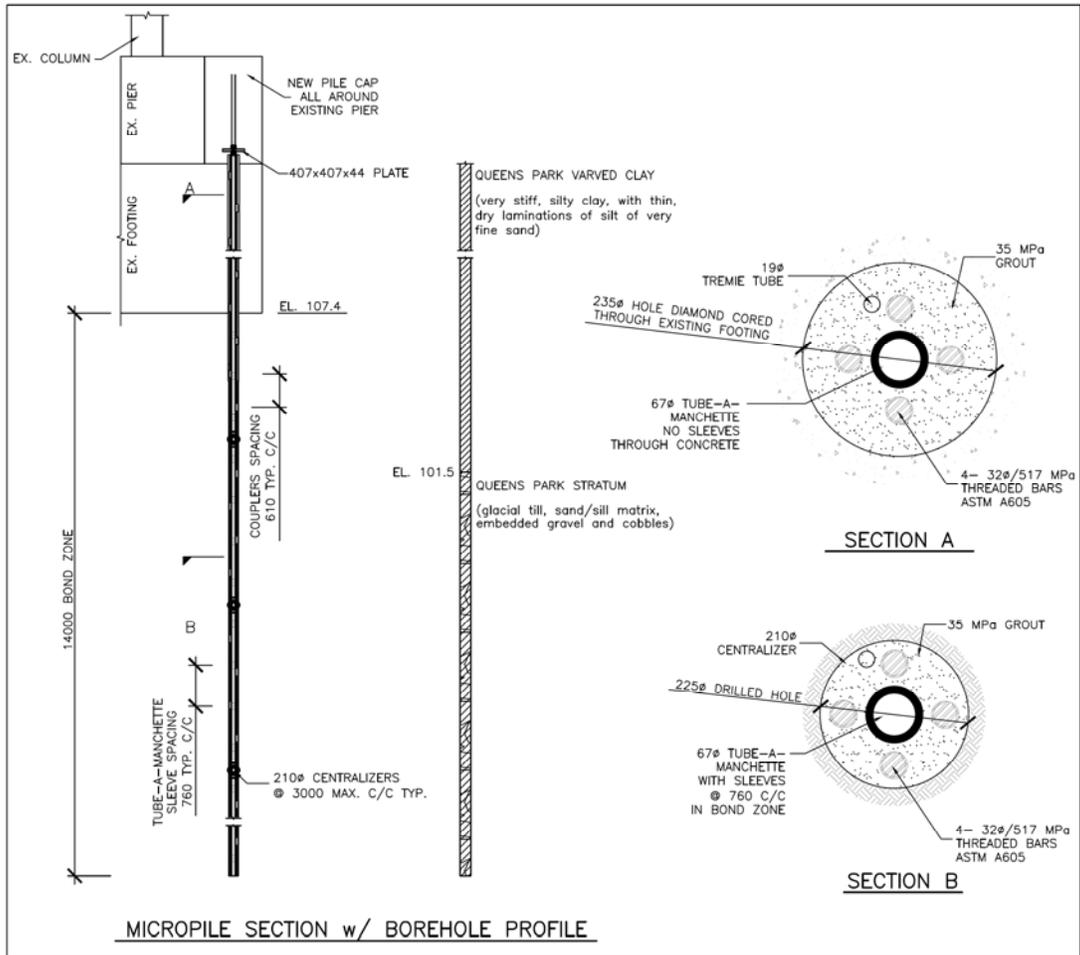
FIGURE 3. 130 Bloor Street West Project - Sub-surface profile and configuration of pre-production micropile
