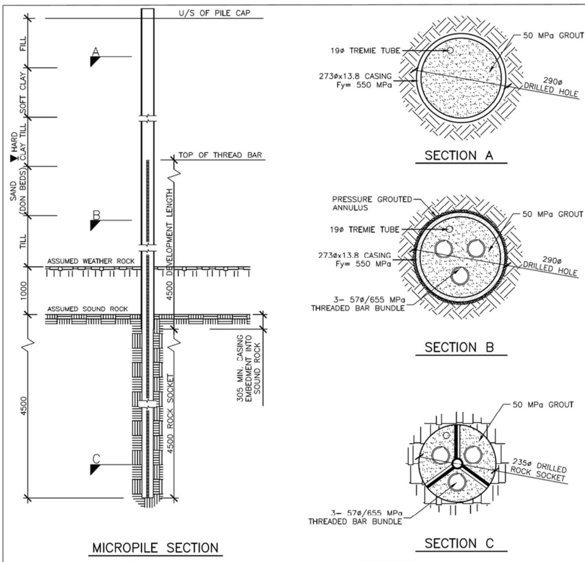
FIGURE 2. Transformation AGO Project - Sub-surface profile and configuration of pre-production micropile
