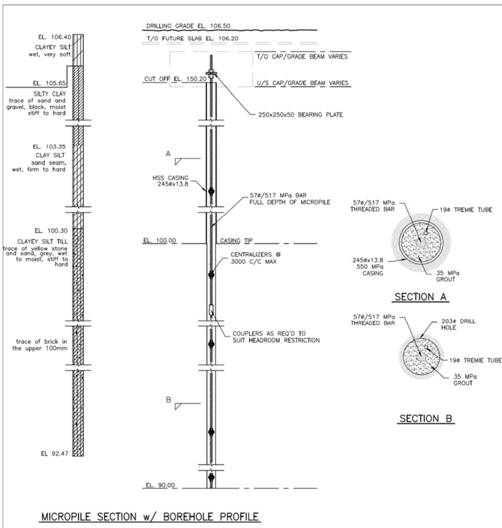
FIGURE 4. Sky Condominium Project - Sub-surface profile and configuration of pre-production micropile
